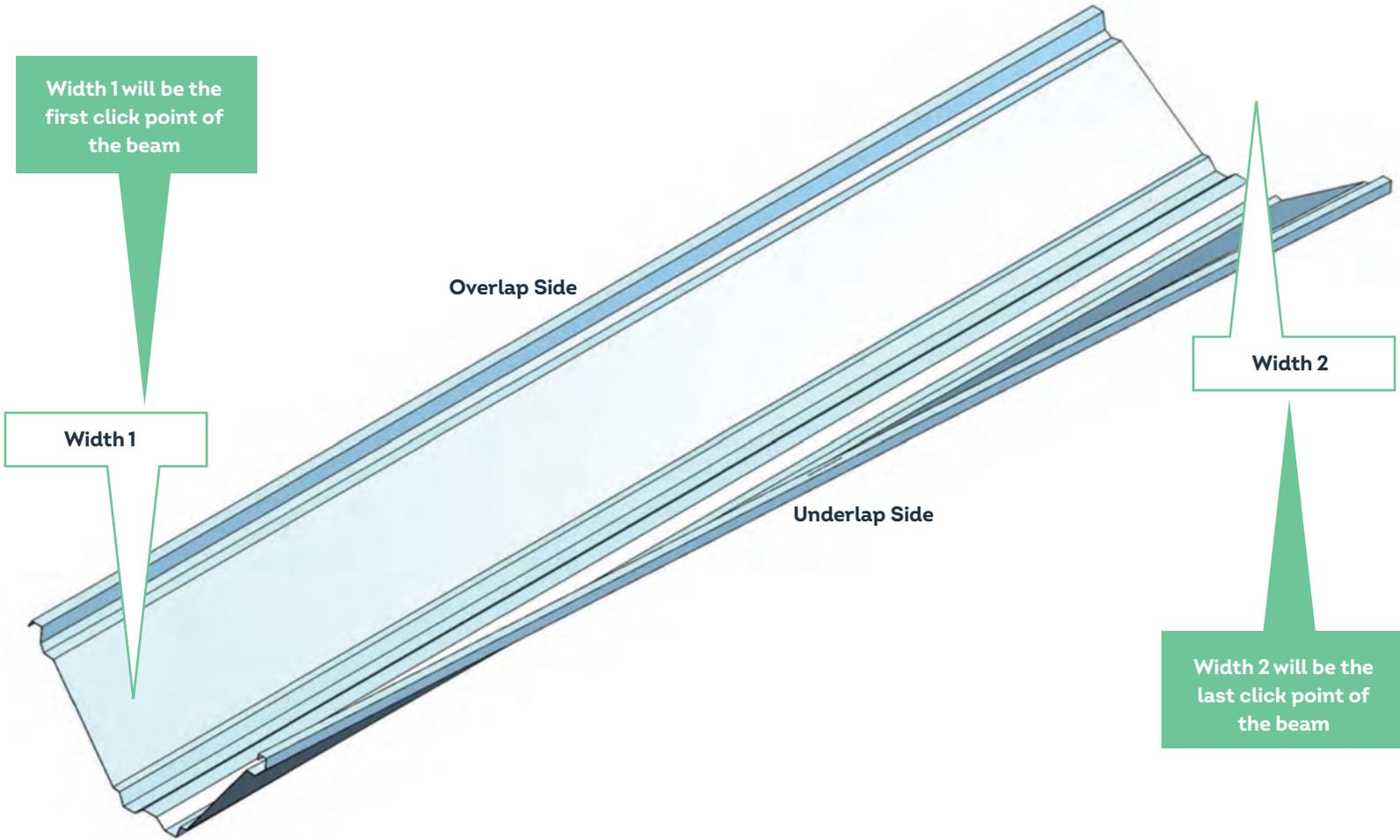
When Equal\_Taper\_Both\_Sides is selected, the user only needs to adjust Width1 and Width2 as desired to achieve an even taper on both Overlap and Underlap sides. Here is a typical example:
