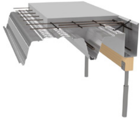
Unsupported edge detail ripped sheet with closure flashing and edge form - propping required
