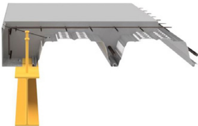
Downstand beam edge detail with SlimDek 210® parallel to beam
