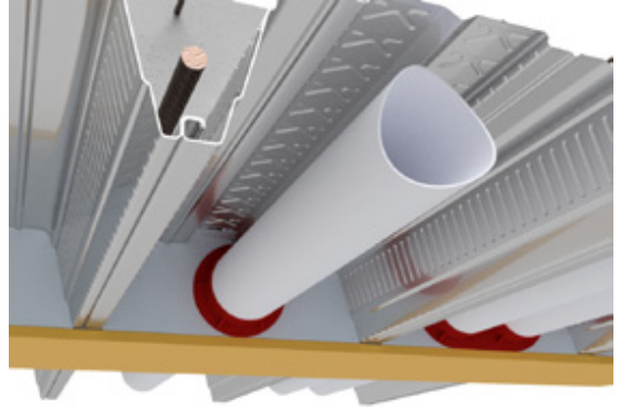
Penetration in ASB with fire collars installed
