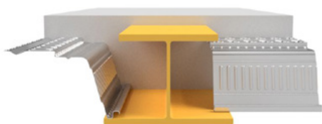
SlimDek 210® supported on ASB with change of SlimDek 210® spanning direction
