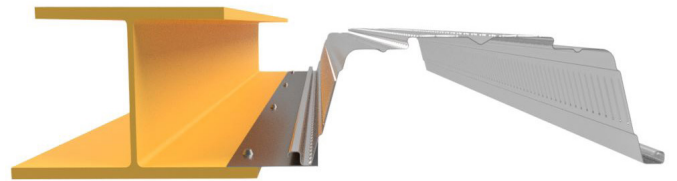
Edge Beam with edge form SlimDek 210™ full sheet parallel to beam with closure plate
