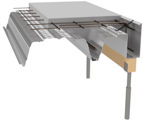
Unsupported edge detail ripped sheet with closure plate and edge form - propping required
